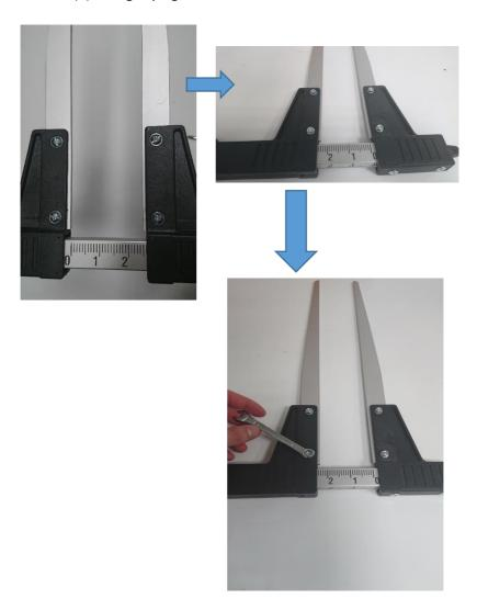
3. Before final tightening, move caliper jaws together to check if they adhere to each other on the entire length.
