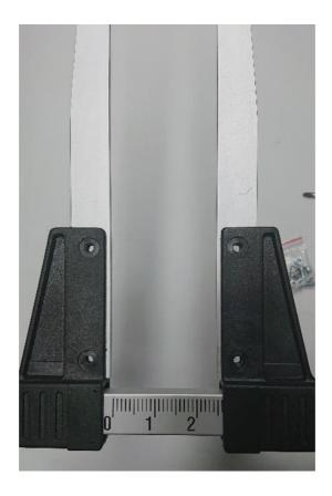
2. After placing the jaws into the plastic bodies, please insert four screws into the drillholes, put the nuts on the screws and use a flat wrench (3) to slightly tighten the nuts.
