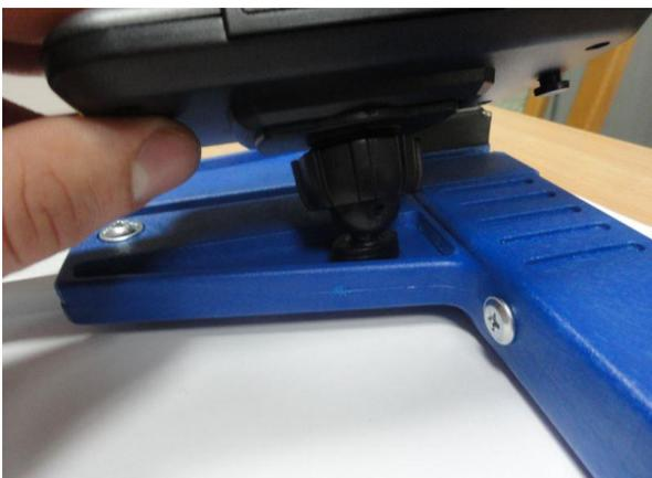
Prepared holder put on a circular element. Set the desired position and tighten the nut to the right to stabilize the handle.
