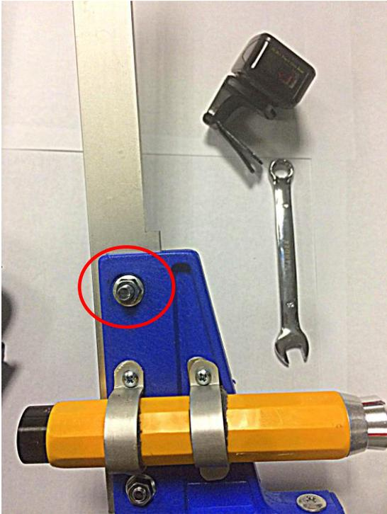
1. With the key number 8 unscrew circled nut (move left). Replace the unscrewed screw from the caliper for longer, included in kit with scanner.
