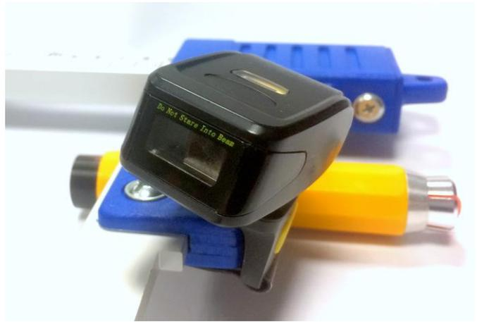
The advantage of using a barcode scanner is the ease of use, simplicity and speed of entering next numbers in single piece measurement method.
