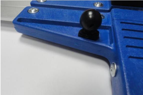
Part of the holder is bolted to stable jaw of calliper by screw.
