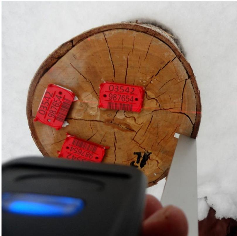
The scanner reads very well barcodes on wood marking tags produced also by Codimex company.
