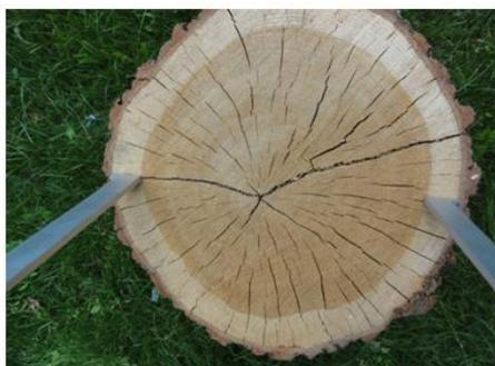
Measurement of the diameter is made by placing the diameter jaws in front of the log on the shortest diameter (bypassing the thickness of the bark). Then by pressing the "▶" button on the caliper the measurement is sent via Bluetooth to the "Log-caliper" application installed on your smartphone or tablet.
