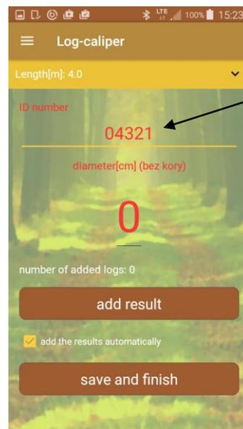
2. First enter the ID number (manually or using the scanner). Next send result of log diameter by pressing button "►" on caliper, or enter manually from smartphone keyboard. After manual adding always click „add result”
