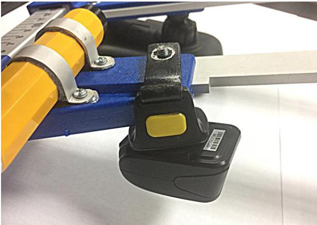
2. On the replaced screw install the scanner mounting bracket as shown in the picture (view from below). Then move nut to the right to stabilize the handle.
