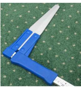
The caliper's body is made of high durability plastic material that is also resistant to washing by means of solvents (such as gasoline, acetone).
