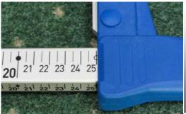
The shape of fixed handle enables to easily slip the caliper under the lying logs in order to make measurement.
